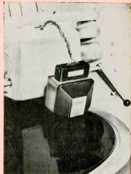
The Ortofon DSS601, an example of a modern stereo cutting head.
